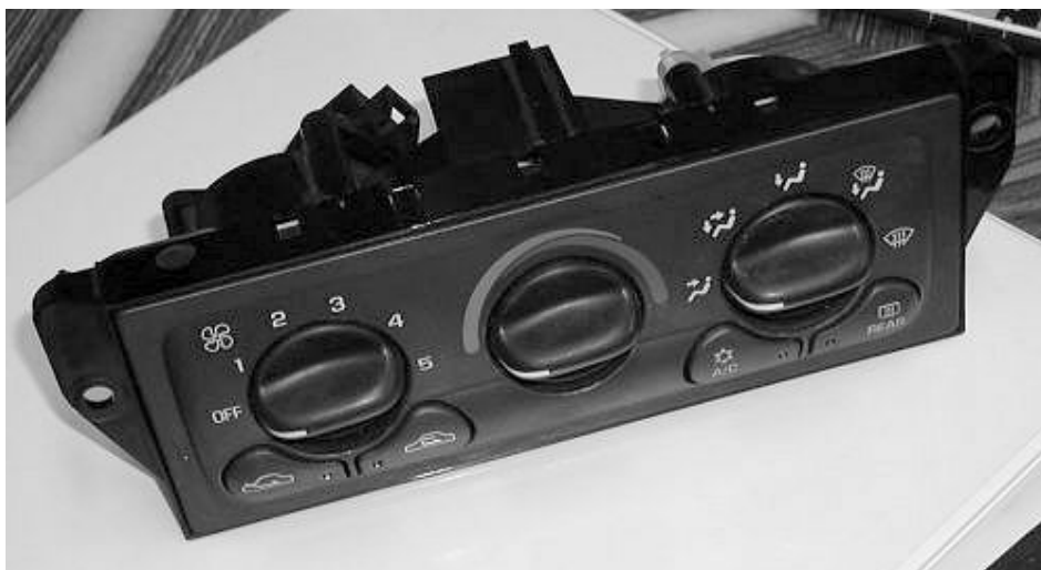
Above: Photo 2. Control Head removed. This unit is probably suffering from dirty contacts. With proper technique, this part can be restored to a servicable condition and live for several years.
