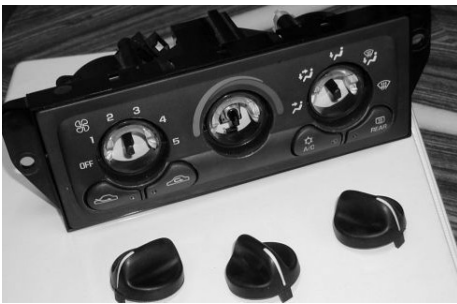
Photo 3. Remove the knobs from the Control Head.
