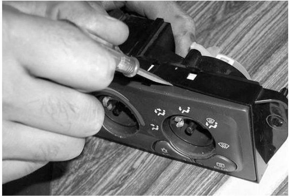
Photo 4. Gently pry the face off of the Control head. Here we are using a small screw driver.
